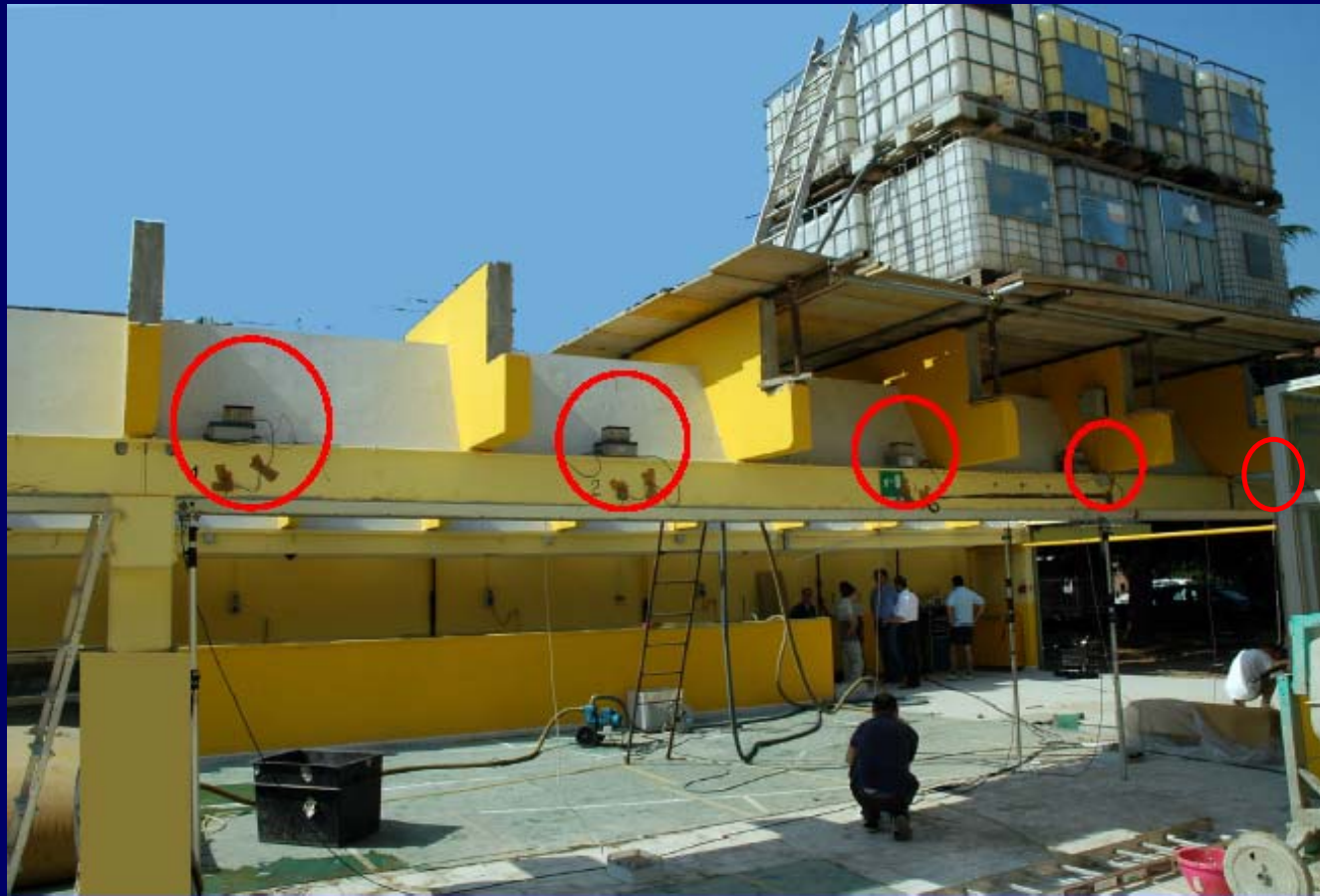
Loading test with AE sources localization
