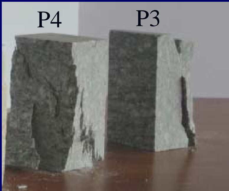
Specimens P3 e P4 in Luserna granite following compression failure.
